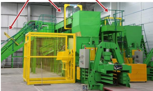
3 conveyors protected by 1 Guardian
